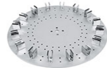
Cat. No.: 18900161 Type 2 plate 16*15ml centrifuge tube
